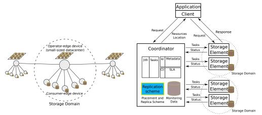
Fig. 1. Storage Elements (SEs) and Storage Domains (SDs)
