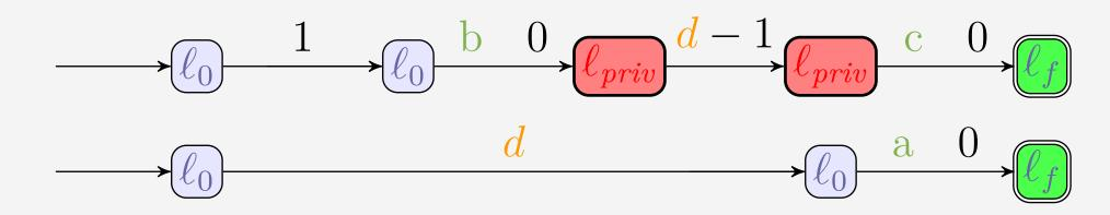
The system is **opaque w.r.t.**  $\ell_{priv}$  on the way to  $\ell_f$  for all durations in [2,3] • But it is not possible to reach  $\ell_f$  with a path of duration 1.5 not passing by  $\ell_{priv}$ The system is **not** fully opaque w.r.t.  $\ell_{priv}$  on the way to  $\ell_f$
