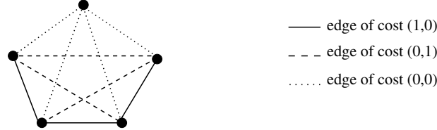
Figure 5.2: Graph for which there is no (1/3 + \epsilon) approximation of the ideal point. Solid edges are of cost (1, 0) , dashed edges are of cost (0, 1) , dotted edges have cost (0, 0) .
