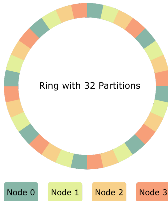
Figure 3.: Structure of the Riak Core Ring
