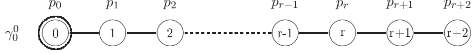
Figure 2: Initial configurations used in the proof of Proposition 4 (the numbers represent clock values and the double circles represent crashed processors).
